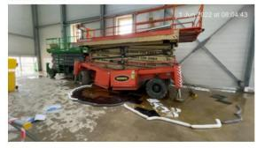
The type of MEWP involved is a HOLLAND LIFT model type: HOL-M250DL27, a technical investigation is underway as well as a full investigation into this serious incident. Findings from both will be analysed and lesson learnt communicated. Immediate actions for project and site managers are: -
